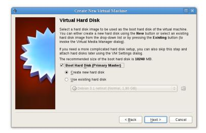
The wizard allows you to create an image file or use an existing one. Note also that the disk images can be separated from a particular VM, so even if you delete a VM, you can keep the image, or copy it to another host and create a new VM for it there.
