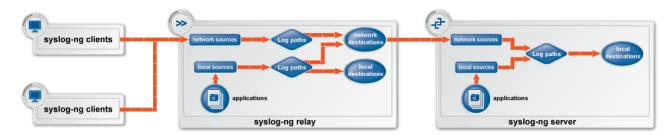
Figure 2.3. Relay-mode operation
