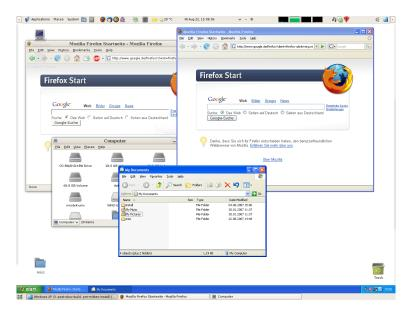
To enable seamless mode, after starting the virtual machine, press the Host key (normally the right control key) together with "L". This will enlarge the size of the VM's display to the size of your host screen and mask out the guest operating system's background. To go back to the "normal" VM display (i.e. to disable seamless windows), press the Host key and "L" again.
