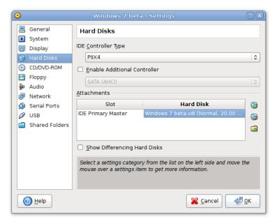
As with a real PC, VirtualBox by default offers you **two IDE controllers**, each with a "master" and a "slave" connection. With one of these four connectors being reserved to the CD-ROM/DVD drive (see below), that leaves you with three possible hard disks, each represented by one disk image file.
