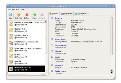
On the left, you can see a pane that lists all the virtual machines you have created so far (quite a few in the example above). A row of buttons above it allows you to create new VMs and work on existing VMs. The pane on the right displays the properties of the virtual machine currently selected, if any.
