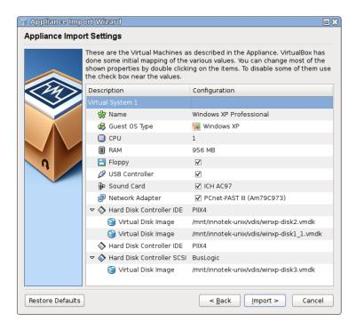
This presents the virtual machines described in the OVF file and allows you to change the virtual machine settings by double-clicking on the description items. Once you click on "Import", VirtualBox will copy the disk images and create local virtual machines with the settings described in the dialog. These will then show up in the list of virtual machines.
