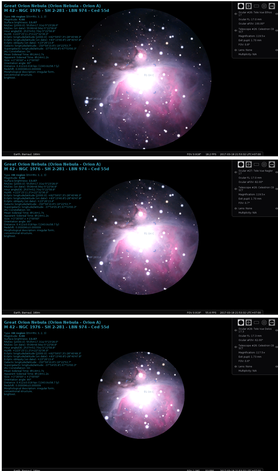
Figure 15.17: Comparing apparent fields of view of (top) a 17 mm Tele Vue Ethos eyepiece with an aFOV of 100°. Magnification is 119.5×. (center) a 17 mm Tele Vue Nagler eyepiece with an aFOV of 82°. Magnification is 119.5×. (bottom) a 17.3 mm Tele Vue Delos eyepiece with an aFOV of 62°. Magnification is 117.5×.
