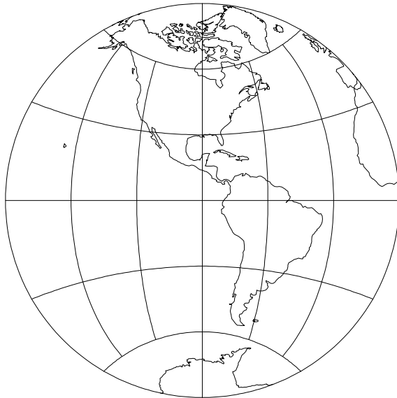
Figure 62: Fournier Globular I projection, with shorelines and 30° graticule. Central Meridian 90° W ( +proj=fourn +lon_0=90w ).
