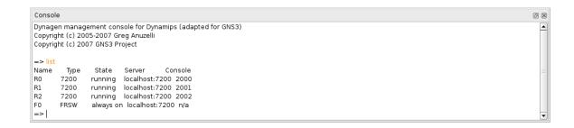
The Frame Relay switch F0 is listed, but you can't stop, start, suspend, or resume it like you can with virtual routers.
