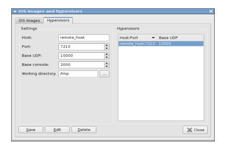
Here we recorded a new hypervisor which will listen on port 7210 on the "remote\_host" machine. You can also specify the fully qualified path to the working directory where the hypervisor will store all of its generated files on the Dynamips host. Be sure to use the correct directory separation character for the platform (here forward slashes for a Linux system).
