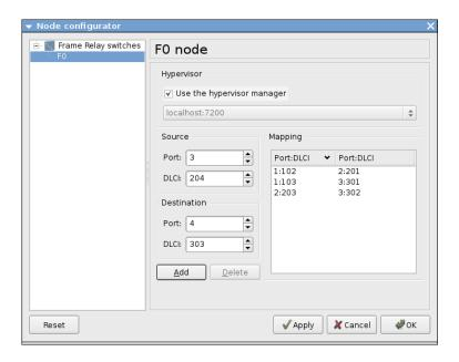
Through the Node configurator we assigned a local DLCI of 102 on port 1, which maps to a DLCI of 201 on port 2. The other two entries are configured similarly, thereby creating a full mesh of PVCs between the three routers. (103 <-> 301, and 201 <-> 302).
