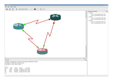
Once connected with by console to your routers, you can assign appropriate IP addresses to the serial interfaces (you can see the connected interfaces by looking at the topology summary on the right or by letting your mouse hover over a link), and "no shut" them, because they are indeed connected.
