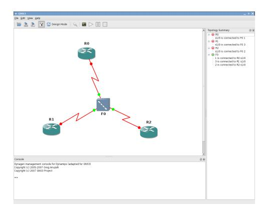
We have connected the routers' serial interfaces to ports 1, 2, and 3 respectively on a Frame Relay switch named "F0".
