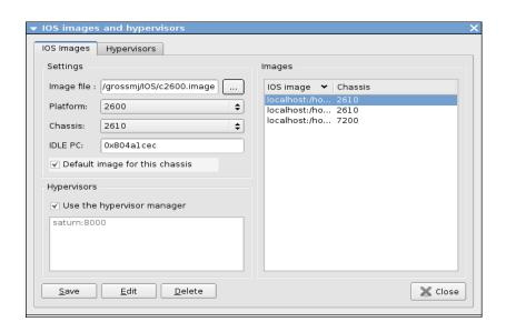
In the following example we created a topology of 3 routers (2610 chassis) and we saved it in emulation mode. A default IOS image for the 2610 chassis has been configured.
