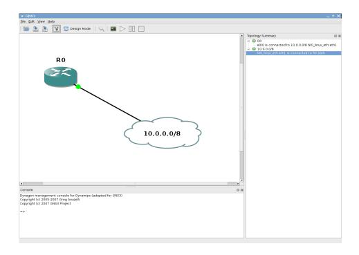
On Windows systems, the Winpcap library is used to accomplish this bridging. The interface format is a little more complex than on Linux systems. GNS3 will perform an auto-detection with the help of Dynamips to list the available interfaces. If the detection did not work, use the shortcut created by the GNS3 Windows installer (thanks to Dynagen). On the desktop, open the "Network Device List" shortcut:
