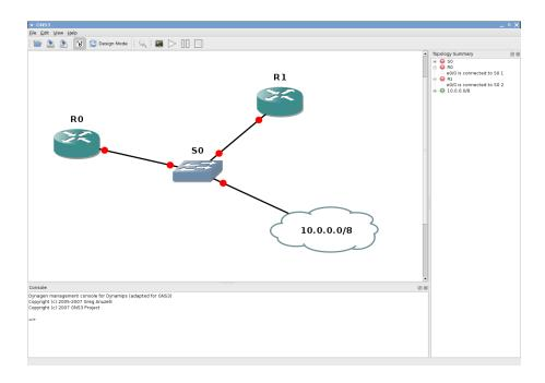
Port 1 of the switch (connected to R1 e0/0) is an access port in VLAN 1. Port 2 is also an access port. Port 4 is a trunk port (specified with the dot1q keyword) with a native VLAN of 1. Trunk ports trunk all the VLANs known to the switch.
