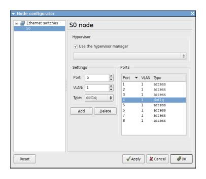
By default in GNS3, a switch has 8 access ports configured in VLAN 1.
