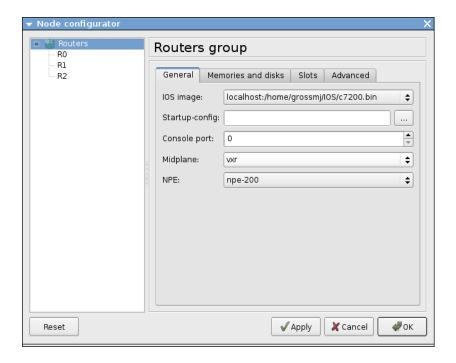
In the node configurator you can select the IOS to use and configure many other things like the startup-config, the RAM size, the slots etc.
