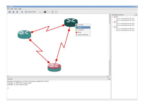
Your network topology with all settings is then created on the hypervisor(s). You can start/stop/suspend an IOS instance by right-clicking on a node. If you have started the IOS, you may also go to a console session for the device. Note: multiple nodes may be selected in order to perform the operation on those nodes at the same time.
