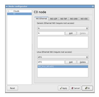
Then you can connect your cloud to a router or a Ethernet switch. In the following image we bridged the router's e0/0 interface to the eth1 interface on the host. Packets that exit e0/0 are dumped out onto the real network through eth1, and return packets are forwarded back to the virtual router instance accordingly.
