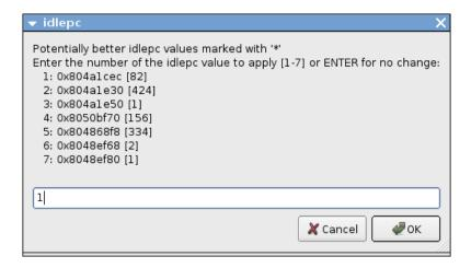
Values that will most likely provide better results are marked with an asterisk. Select one of the values to try from the menu and press the OK button. You should notice your host (the one running the dynamips process) CPU utilization drop dramatically. If so, you've found a good idlepc value for this particular IOS image.
